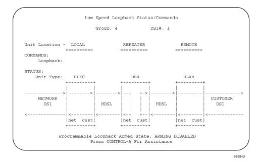
Figure 541-8a. HRX Customer Loopback Screen (One HRX)
